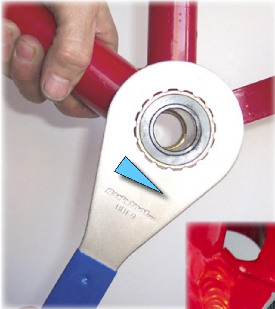
5) Remove the left, or non-drive side bearing cup.
