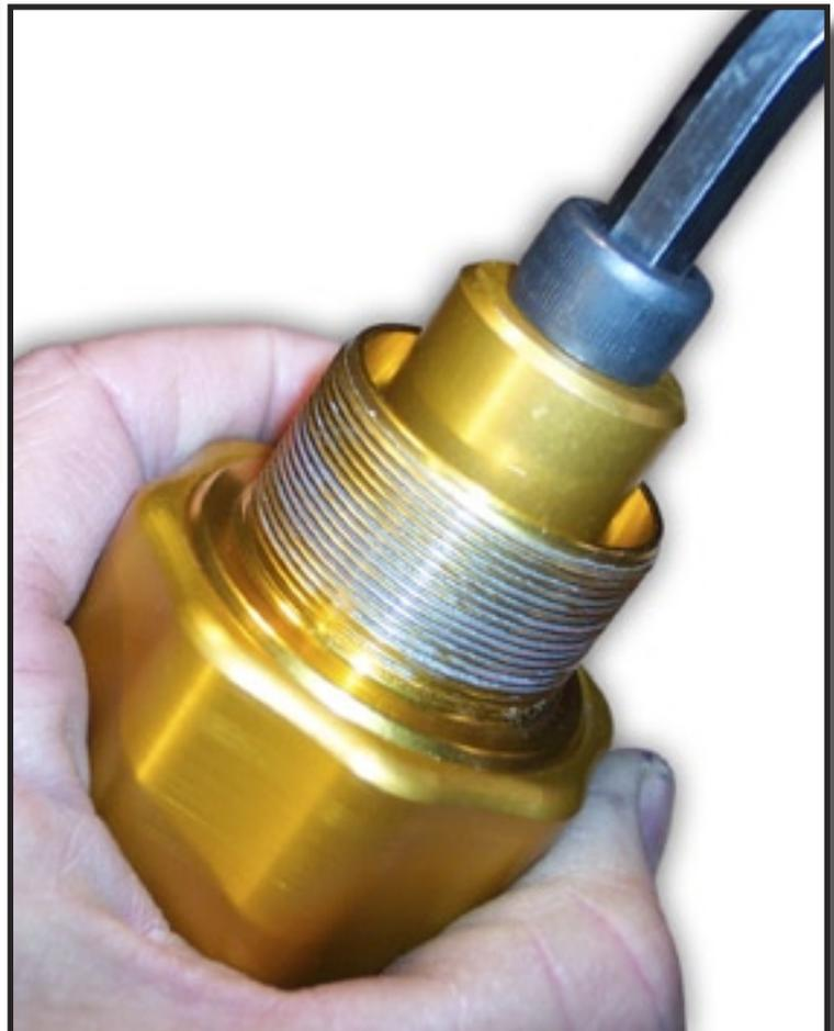
11) Press out the bearing and plastic cap by inserting the Bolt and using an 8mm Allen wrench to turn it clockwise until you hear and feel the bearing “drop out” of the cup.
