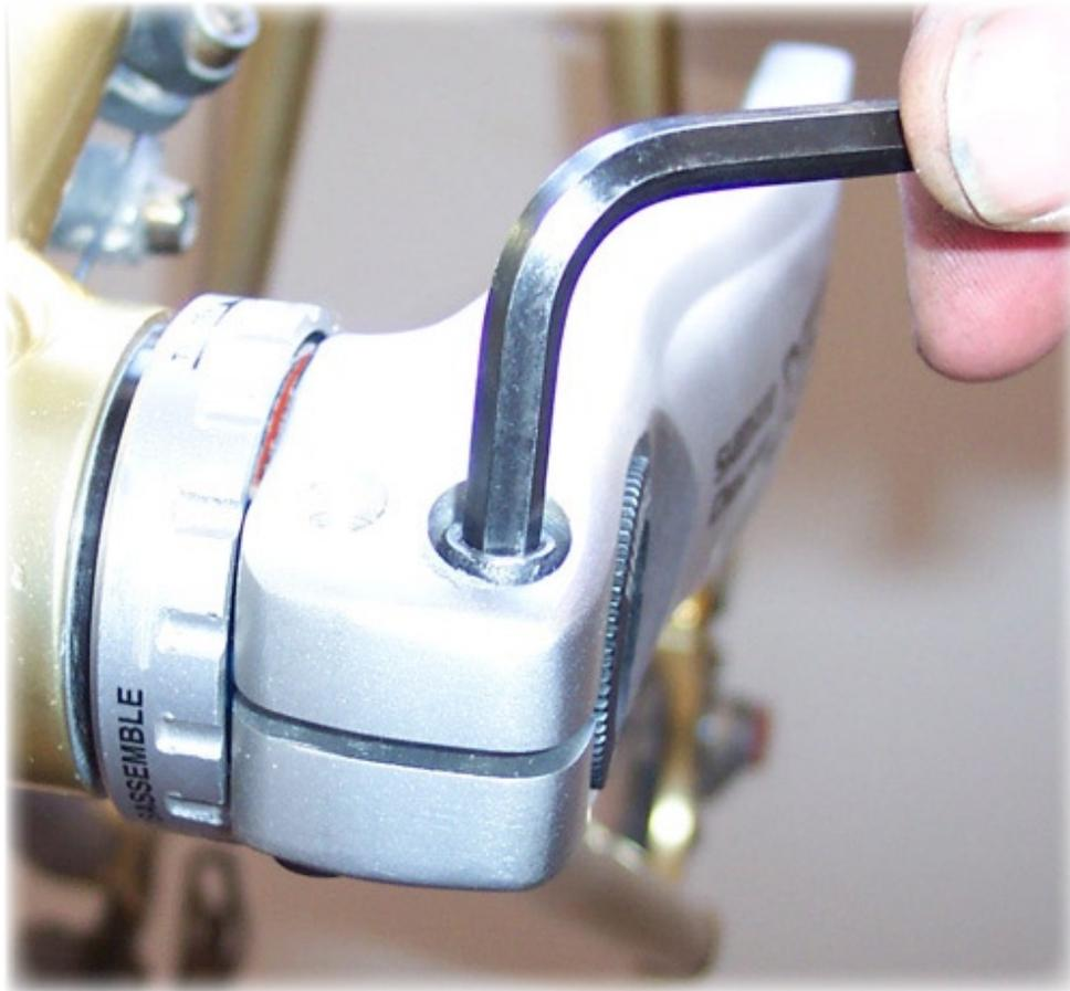
30) Check that there is no side-to-side play (looseness) and that the crankset spins freely and smoothly. If so, put your chain back on and hit the dirt!
