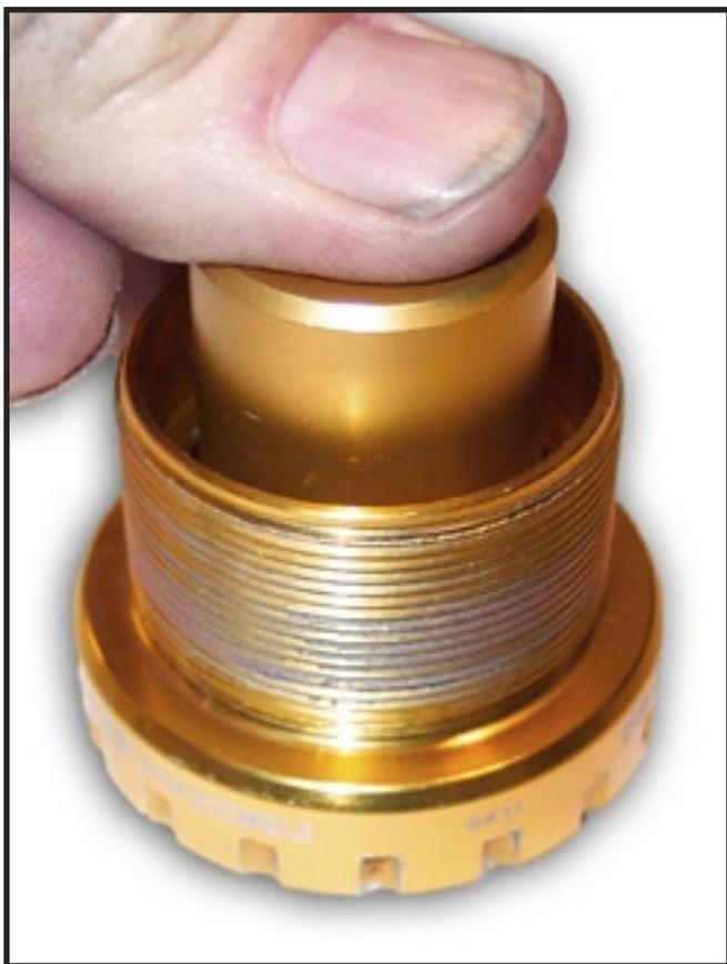
9) Apply pressure to the Collet Expander until it “seats” between the collet halves.
