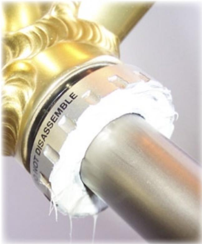
25) Insert the right crank assembly. If your bike's bottom bracket faces are parallel and the bearings are properly seated, the spindle should line up with the opposite bearing and come through with very little effort. If the spindle tightens up at the last few millimeters, you may lightly tap the drive side with the rubber-faced mallet.
