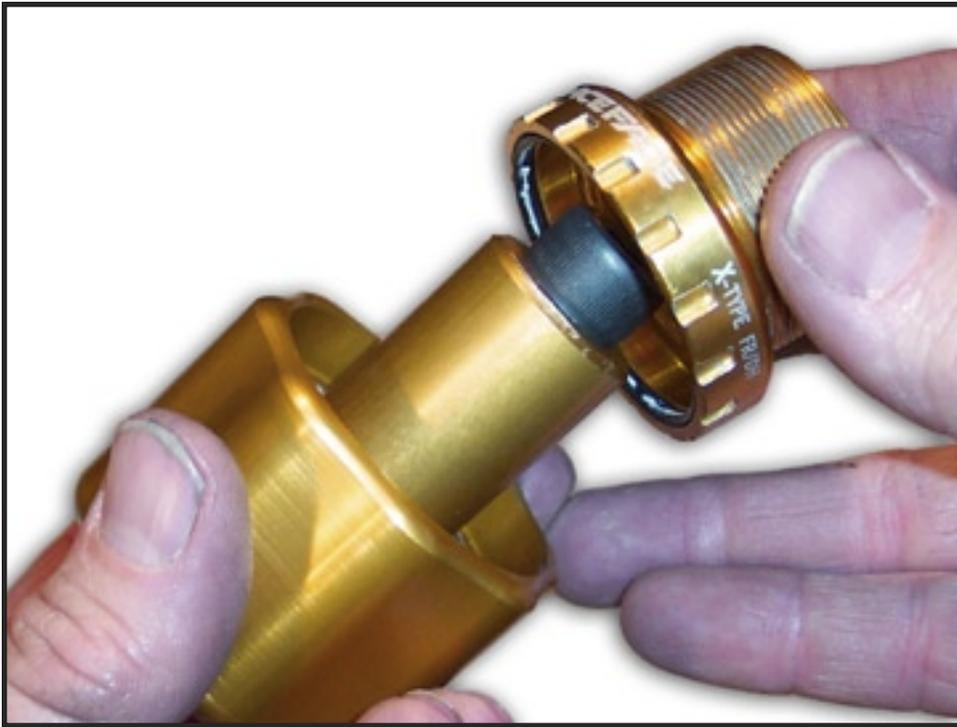
13) Unthread the Bolt from the Cup Holder and remove the old bearing and plastic cap.
