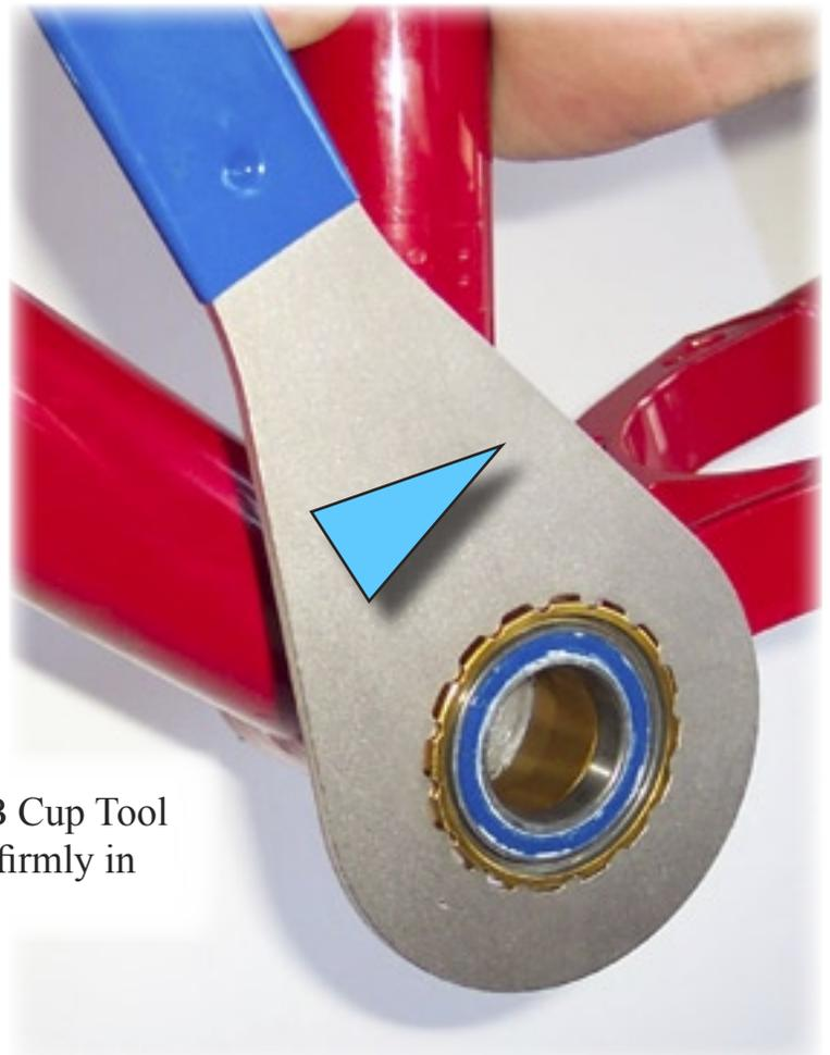
d) Use a proper BB Cup Tool to tighten the cup firmly in place.
