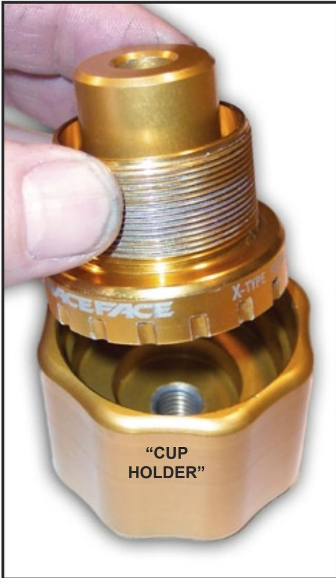
10) Set the bearing cup (with collet and expander) into the Cup Holder.
