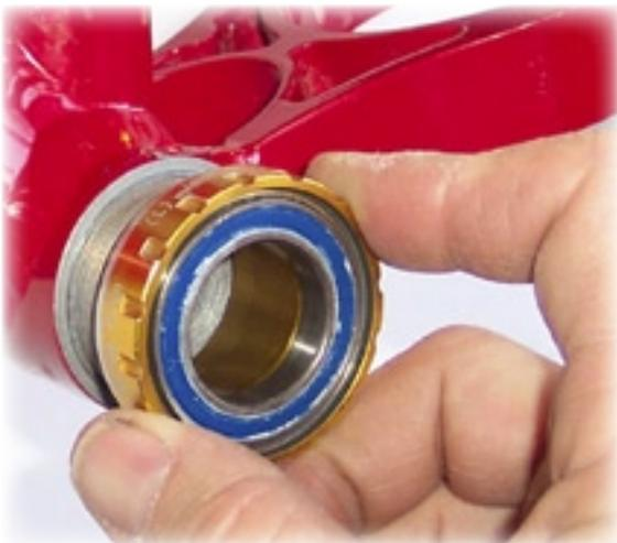
c) Start the cup into the frame by hand. The left side threads in normally (clockwise).
